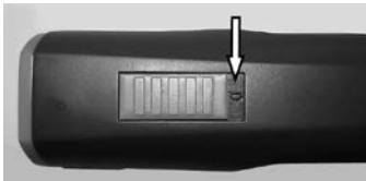
Fig. 4 Switch in OFF-position ("0")
