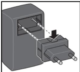
1. Hold down the release key **8** while pulling off the mounted mains plug adapter **9**.
